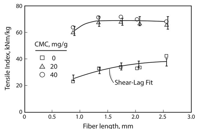
**Figure 6** Tensile strength index versus fiber length for different levels of CMC addition. The curve for the untreated papers is a fit to the shear-lag model.
