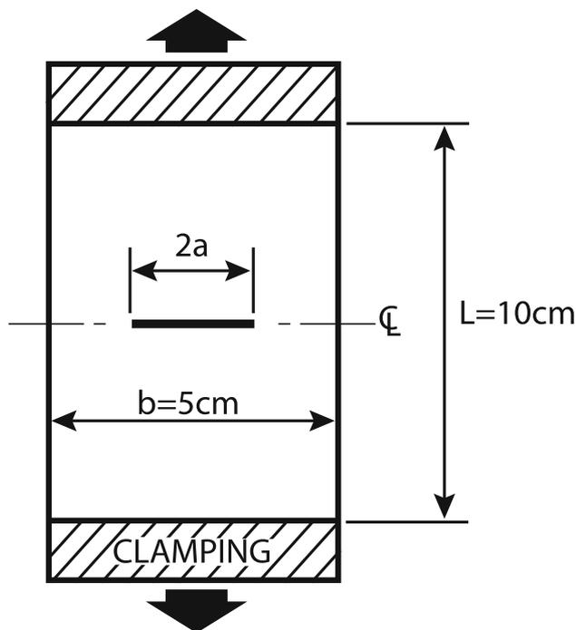
**Figure 2** Center-notch specimen for fracture testing.
