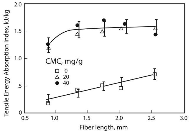
**Figure 8** Tensile energy absorption index versus fiber length for different levels of CMC addition.
