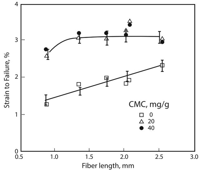
**Figure 7** Strain at break versus fiber length for different levels of CMC addition.
