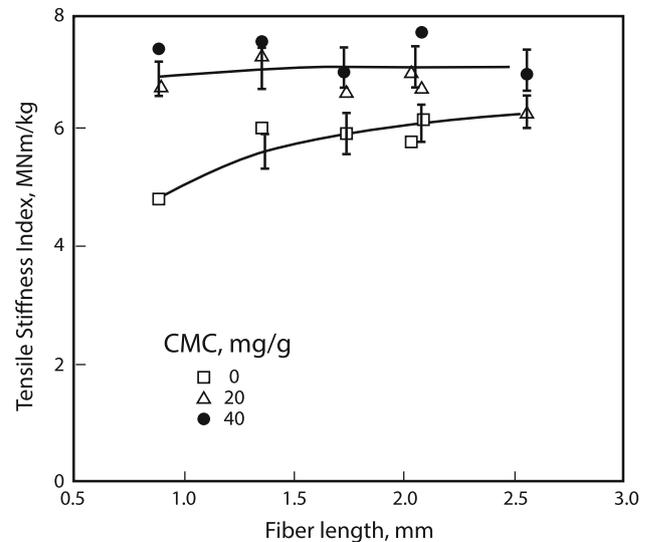
**Figure 5** Tensile stiffness index versus fiber length for different levels of CMC addition.
