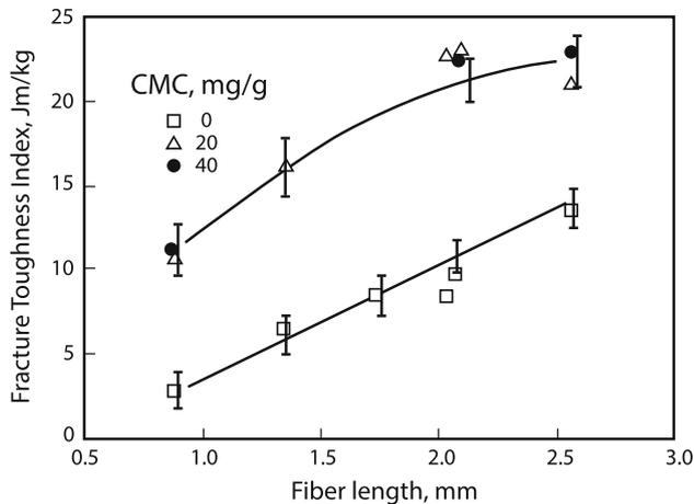
**Figure 9** Fracture toughness index versus fiber length for different levels of CMC addition.
