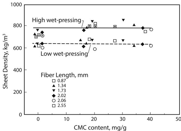
**Figure 4** Sheet density versus CMC content for different fiber lengths. Results are shown for two wet pressing levels.
